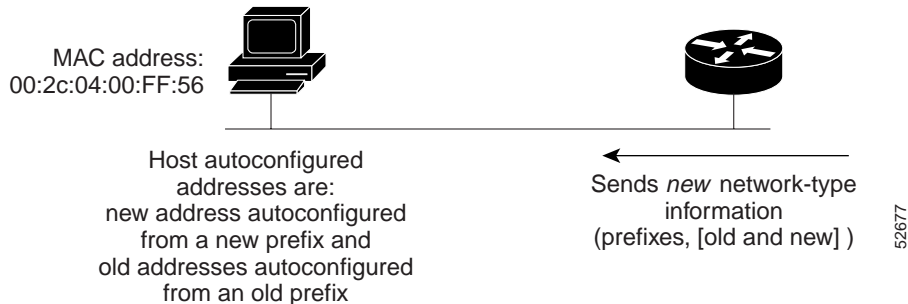
Figure 17 IPv6 Network Renumbering for Hosts Using Stateless Autoconfiguration
